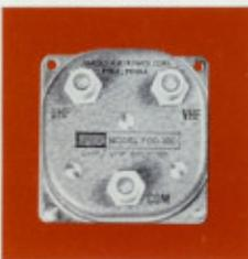
FREQUENCY RANGE: 470 to 890 MHz. BANDWIDTH: 6 MHz. MAXIMUM VSWR: 1.79:1 (minimum return loss of 11 dB). IMPEDANCE: 75 ohms input and output. INSERTION LOSS: 1 dB. OUT-OF-BAND REJECTION: 19 dB.
