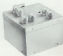
Model UMN-3 contains 3 cavity-type, double-tuned filter networks which allow guardbands of 2 channels at low-end, 3 channels at mid-band, and 5 channels at the high end. It may be ordered factory-tuned to specific channels. It is designed for either indoor or outdoor mounting.
